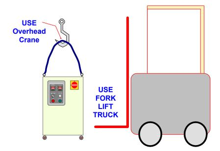
Figure 3: Suggested Lift Rigging for Cart Mounted Dryers
